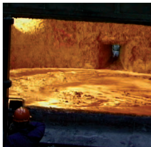
Bath homo- genization by use of stirring technology
