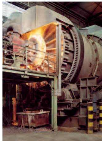
Slag cleaning furnace at AURUBIS - Lünen Plant/Germany
